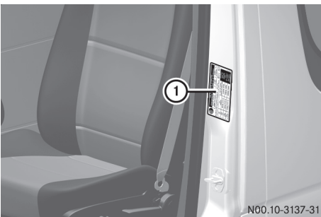
Example: Tire and Loading Information placard on the B-pillar, driver's side
